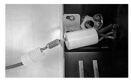
Disconnect the metal locking connectors by squeezing the metal tab.
